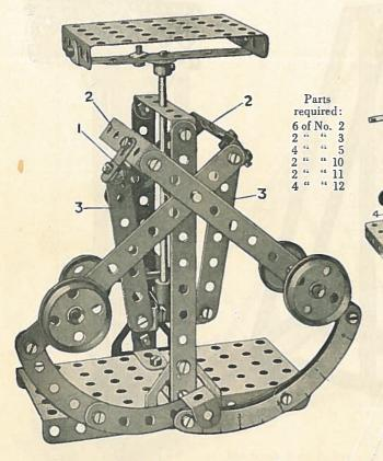
The connection at (1) of the rocking arms (2) to the thrust strips (3) is locknutted to give a free pivotal action, and similarly the pivotal connections (5) of the strips (3) to the lever strips (4) are locknutted to give free play.
