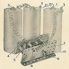
one-way motor in motion. Insulated copper bell wire is recommended for making the connections and can be obtained at any electrical supply store.
