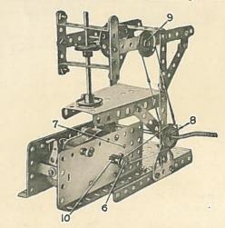
cause it is a great deal larger. However, although the speed of the second shaft is only about 1/5th the speed of the first shaft, it has about five times the
