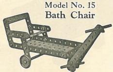
Parts | 1 of No. 16 | 13 of No. 37 required: 2 " " 17 | 1 " " 44 2 of No. 2 | 3 " " 22 | 1 " " 52 6 " " 5 | 4 " " 35 | 3 " " 60
