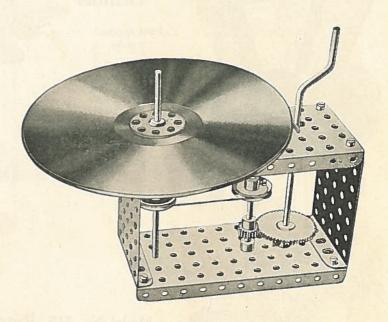
This is a model to show that white light is made up of the three primary colours—red, yellow, blue. Sectors of these three colours are mounted or painted on the disc, which if then quickly rotated, shows as white.
