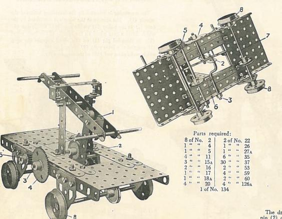
The car is caused to travel by working the rocking lever (1) which is connected by a strip (2) to a crank shaft (3) and a gear wheel (4) meshing with a pinion (5) on a rod coupled by a cord (6) to an axle rod (7) of the travelling wheels (8).
