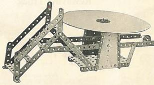
The driving mechanism and construction of the framework of this model are clearly brought out in Fig. 206a. Cut out a circular piece of cardboard, 8" in diameter, and in the centre of the disc fix a bush wheel by nuts and bolts. The eye of the bush wheel is then threaded over the top of a vertical spindle, and secured by its set-screw.
